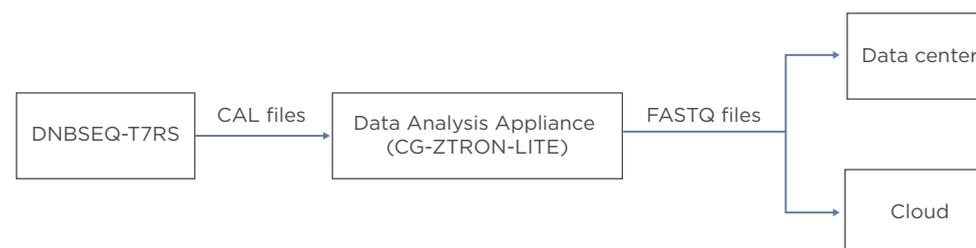
If CG-ZTRON-LITE server is deployed and connected to the sequencer, ZLIMS will monitor the status of the sequencer.
